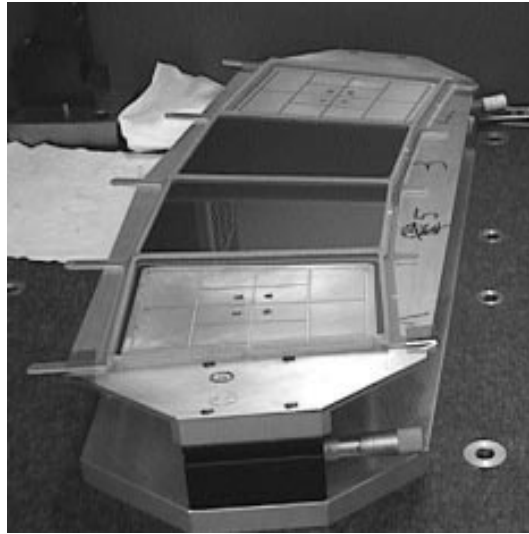
Figure 4: Aligned substrates on the glueing jig.
