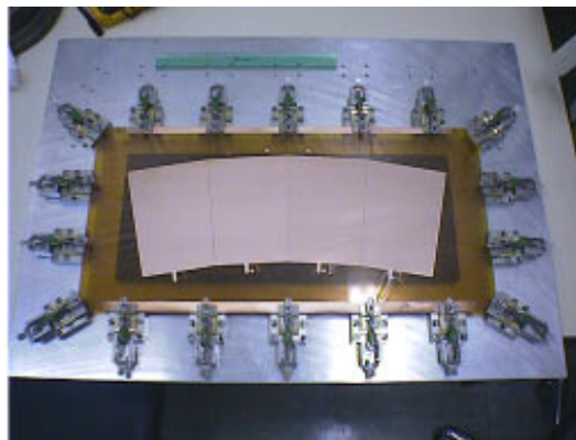
Figure 5: GEM stretched by means of a dedicated tool.
