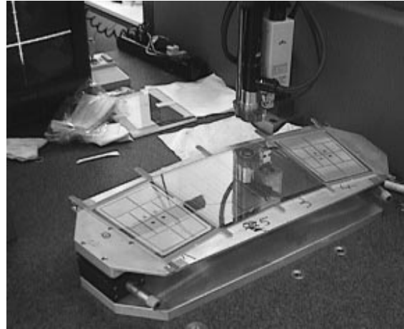
Figure 3: Lower half–module: The substrates are aligned with respect to the support frame. The two outermost glasses are unmetallized dummy substrates.
