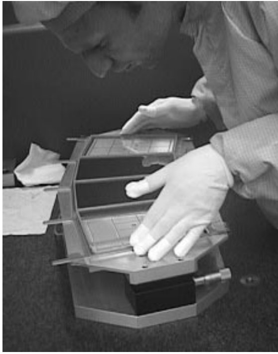
Figure 4: The two half-modules are glued together.
