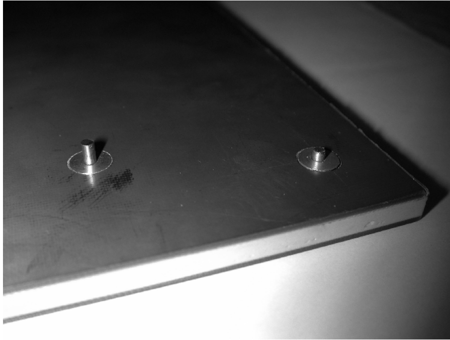
Figure 5 Detail of jig and gap spacers inserted in the polyurethane panel.
