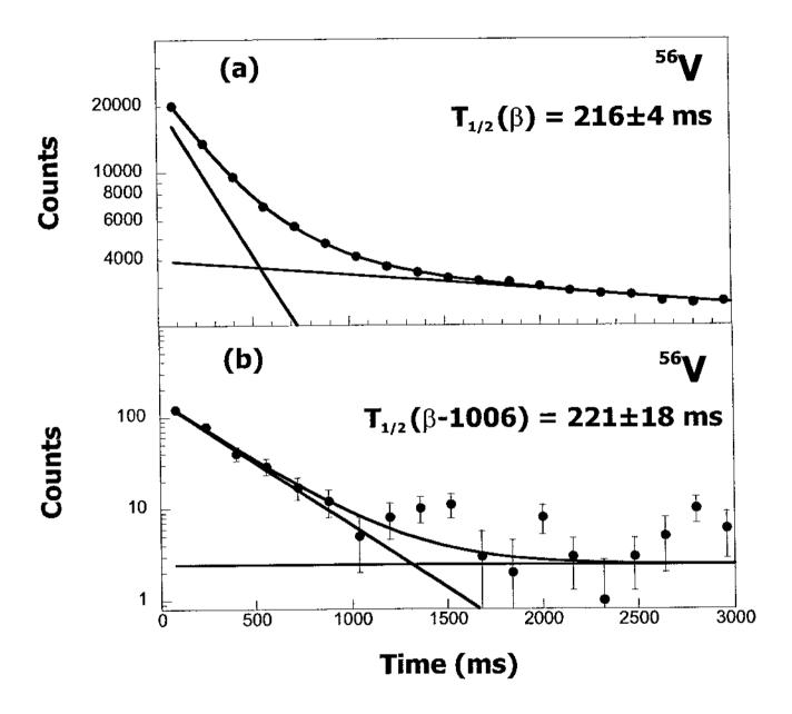
$$\begin{array}{c|c} \hline 1+ & 0 \\ \hline 56V & T_{_{1/2}} = 216\pm4 \text{ ms} \\ Q_{_{\beta}} = 9.05\pm0.24 \text{ MeV} \end{array}$$
