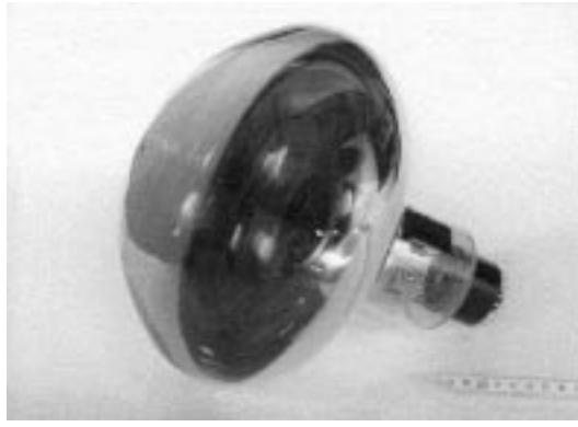
Fig. 5. A 10" photomultiplier model R7081-20 from Hamamatsu.
