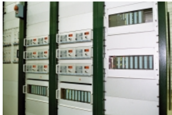
Figure 2: Electronics racks of one high voltage generator showing thyatron heater power supplies, thyatron heater and terminating resistor controllers.
