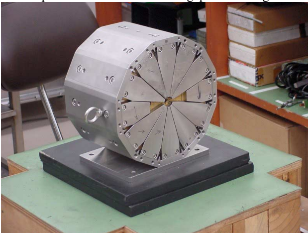
Fig.1 Assembled 4 Tesla permanent magnet
