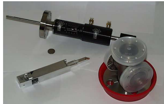
Figure 1: Main components of the intra-undulator diagnostic probe assembly.
