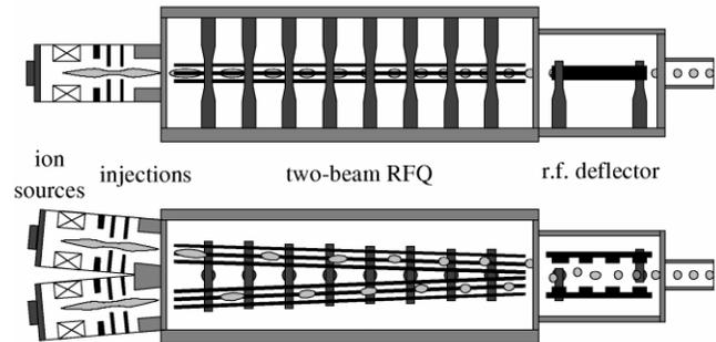
Figure 2: Experimental set-up of the two-beam funneling experiment.
