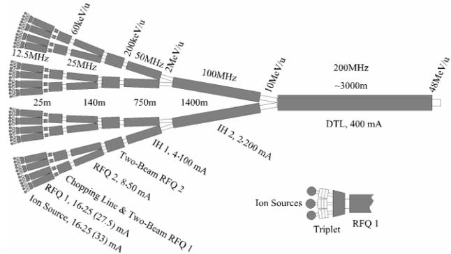
Figure 1: Layout of the 12.5...200MHz linac system for 400 mA of Bi<sup>+</sup>.
