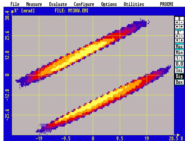
Figure 6: Measured emittances 1m behind the RFQ at the place of beam crossing. The ellipses correspond to the 90% normalized RMS-emittances which are  $\epsilon_{\text{RMS}}=0.107$  and 0.114 mm mrad for each beam.
