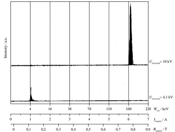
Figure 5: Energy spectra behind the RFQs. With the design voltage of 10 kV the final beam-energy of 166 keV is reached.
