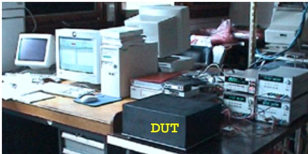
Fig. 9: The automated module test equipment.
