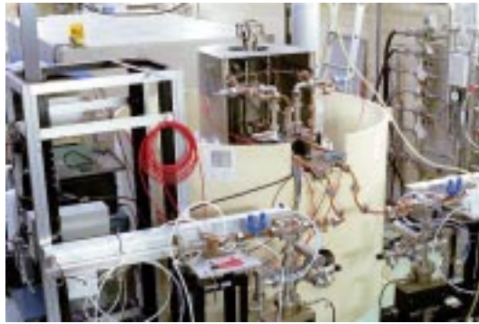
Figure 5.6: Experimental set-up for testing the BINP PPM-2 klystron.
