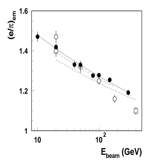
Figure 1: The  $(e/\pi)_{em}$  ratios as a function of the beam energy for this method (black circles) and for weighting method (open circles for Ref. [12] and open squares for Ref. [13]). The lines are the result of a fit of Eq. (3) with free e/h parameter and k=0.11: solid line is for the [23] data, dashed line is for the [12] data and dash-doted line is for the [13] data.
