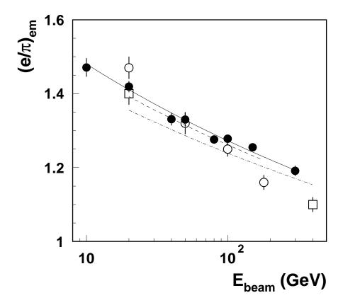
Figure 1: The  $(e/\pi)_{em}$  ratios as a function of the beam energy for this method (black circles) and for weighting method (open circles for Ref. [12] and open squares for Ref. [13]). The lines are the result of a fit of Eq. (3) with free e/h parameter and k=0.11: solid line is for the [23] data, dashed line is for the [12] data and dash-doted line is for the [13] data.
