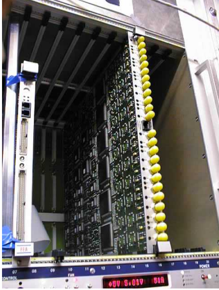
Figure 2: The FLT Track Finding Unit: Ten such 9U VME boards are housed in each crate. In total 74 TFUs are needed.
