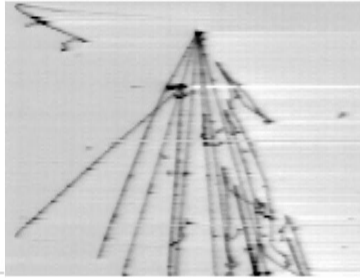
Figure 3: An example of recorded neutrino interaction in the 50 liter Liquid Argon chamber prototype located at the CERN \nu beam. The neutrino comes from the top of the picture. The horizontal axis is the time axis (drift direction) and vertically is the wire number. The visible area corresponds to 47 \times 32 \text{ cm}^2
