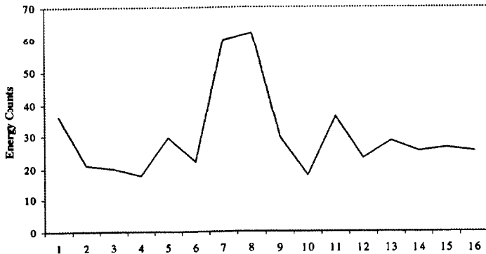
Figure 10. A single Muon event pulse shape vs. time. Note the pedestal noise.
