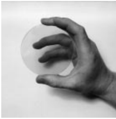
Fig. 1. Free-standing, 100 mm diameter CVD diamond (courtesy of De Beers Industrial Diamond Division (UK) Ltd.) [4].
