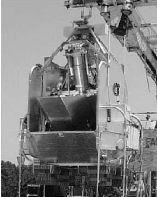
FIGURE 12. Photograph of the MAXIMA gondola shortly before launch. The receiver is visible in the center of photograph. The scoop-shaped aluminum ground shield can be seen, below the receiver. The outside of the gondola is covered with aluminum coated insulation attached to the roll-bars.
