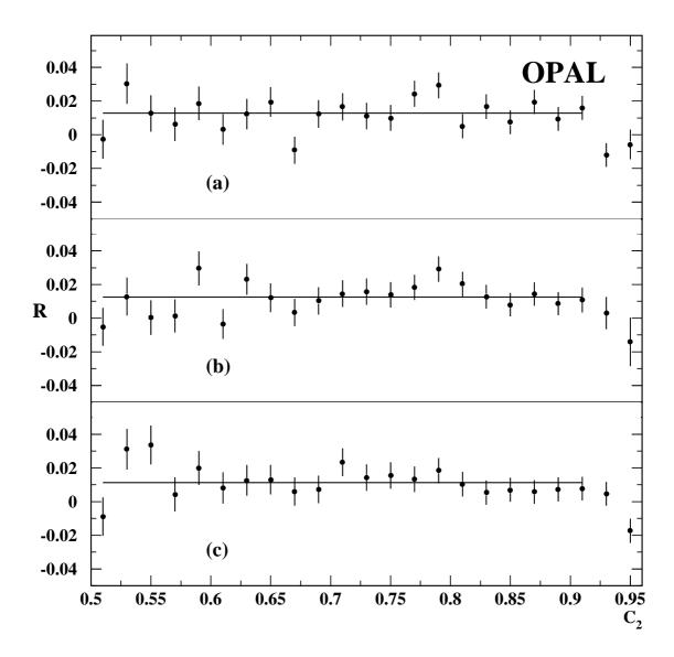
Figure 2: The ratio  $R \approx \sigma_{\rm L}/\sigma_{\rm T}$  for all thrust, computed from pairs of bins in  $|\cos\theta_{\rm Th}|$ ,  $C_2$  being the upper value of  $|\cos\theta_{\rm Th}|$ . The horizontal lines show the average values over the range  $0.5 < C_2 < 0.92$ . Three cases are shown: (a) the standard analysis; (b) tracks alone; (c) calorimetry alone.
