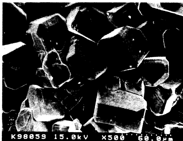
Figure: 2 A SEM photo of cuprite (Cu 2 O) single crystals formed on a damaged stream-forming cylinder made of Cu.
