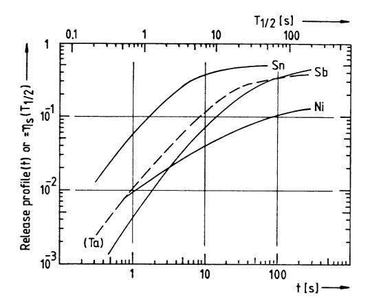
Fig. 2. Release profiles of various relatively refractory elements from FEBIAD-E ion sources [4], catcher temperature 2400 K. Solid lines for sintergraphite catchers, broken line 3  $\mu m$  Ta catcher. The latter measurement is mainly interesting with respect to the considerably faster desorption part of the release which is due to a coating of the inner surfaces of the ion source with pyrolytic graphite here.
