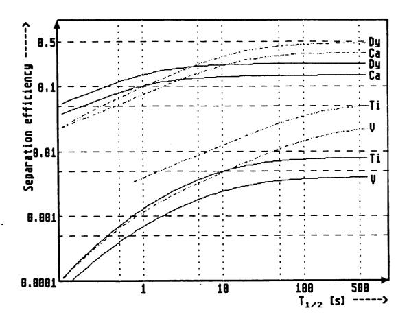
Fig. 3. Halflife-dependence of the separation efficiency of various tracers from 3  $\mu m$  foil catchers in high temperature cavity ion sources [4] at 2700 K. Solid lines: Ta catchers in Ta cavities; broken lines: Re catchers in Re-lined tungsten cavities.
