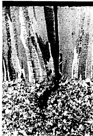
Fig. 21: Micrographs of the hottest tile after the test. The melt layer is up to 0.7 mm deep. Cracks partially penetrate through the melt layer into the base material. Occasionally some of the molten material has flown away.
