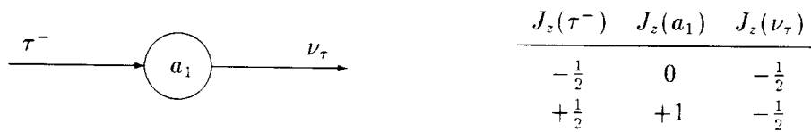
Figure 4.11: Possible spin configurations in the decay (4.28) if the \nu_\tau is left-handed ( a_1^- rest system).
