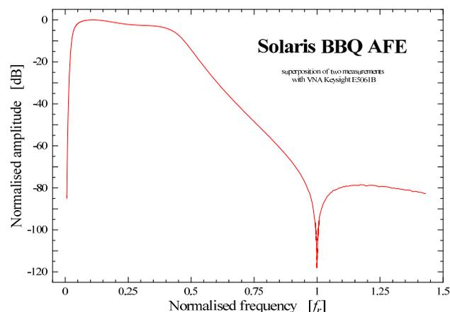
Figure 4: Frequency characteristic of the Solaris BBQ analog front-end.
