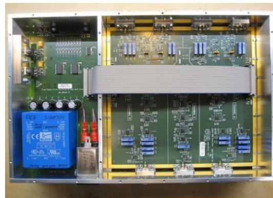
Figure 3: Block diagram of one channel of the Solaris BBQ analog front-end (top) and its photograph (bottom).
