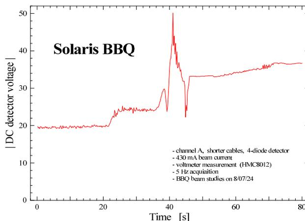
Figure 7: An evolution of the detector DC voltage during bunch length manipulation at the end of the energy ramp.
