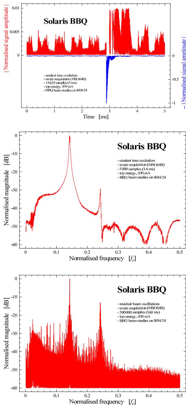
Figure 5: Top: An oscilloscope record of the smallest tune excitation showing the whole rectified signal (blue) and the lowest 1 % of the rectified signal, revealing the residual beam oscillations. Middle: spectrum of the excited beam oscillations shown in the top plot. Bottom: spectrum of the residual beam oscillation prior to the beam excitation in the top plot.
