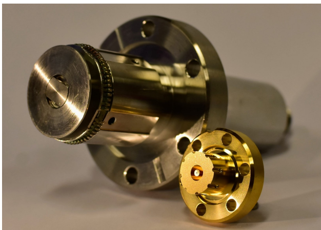
Figure 2: An LEP button type BPM (left) with a cutoff of around 3 GHz, and the HF BPM (right) with a cutoff at 40 GHz.
