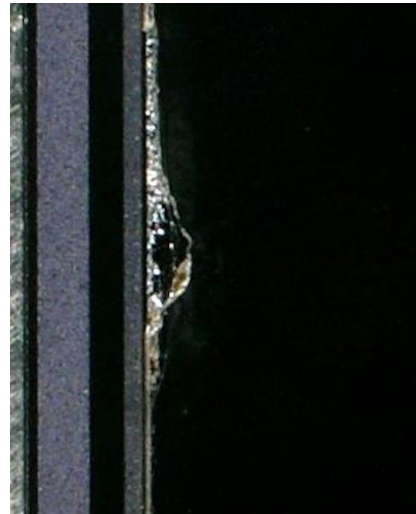
Visual Inspection of an ITkPix v1 module in Milan showing a chipped ASIC border
