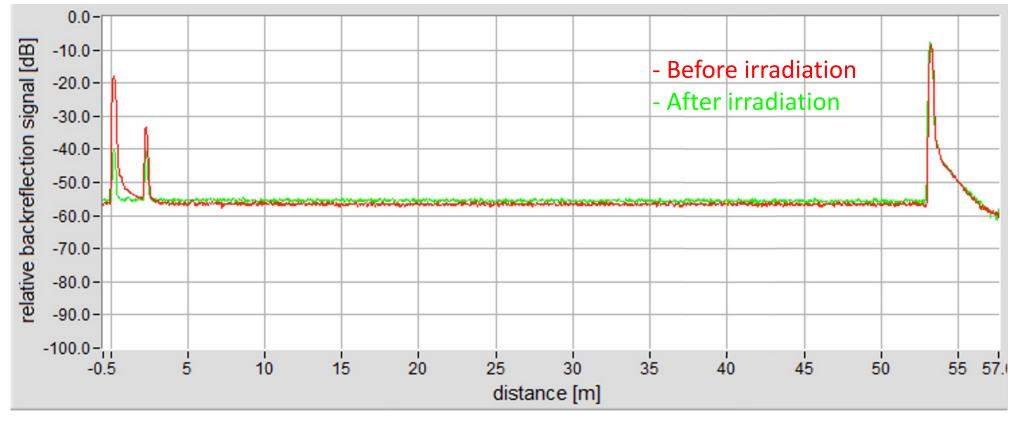
The data obtained with the OTDR (optical time domain reflectometer) show no significant attenuation effect on the optical fiber after the CHARM (CERN High Energy Accelerator Mixed Field Facility) irradiation period, corresponding to 147 Gy of received dose. Based on this result, these fibers meet the total integrated dose requirements equivalent to ten years of HL-LHC operation, 10-12 Gy, with a safety factor close to 15.
