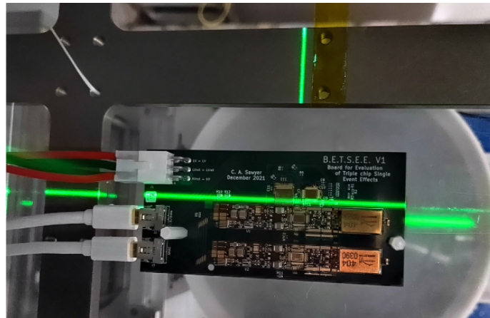
Figure 1. BETSEE board mounted to platform during proton beam running. The green lines shows the rough location of the beam spot with the AMAC, ABC, and HCC inside.
