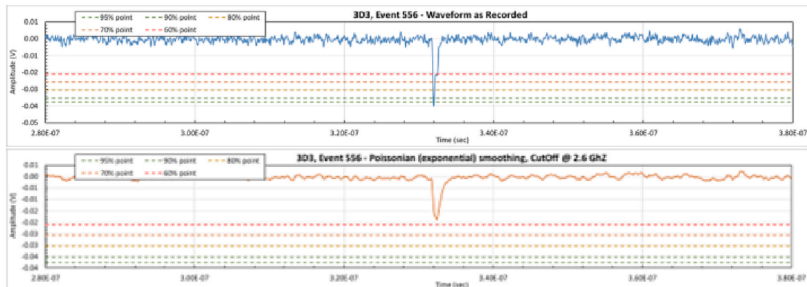
Fig. 8. As recorded and after a 2.4 GHz Gaussian filter 3D signal. Dotted lines indicate percentages of the original signal amplitude.
