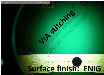
Figure 1: VIA stitching and surface finish implemented on the VFE card.
