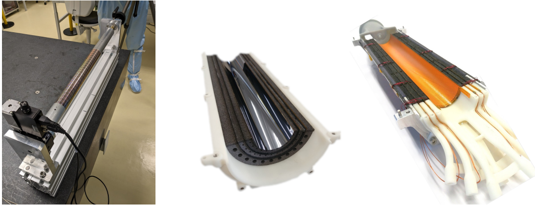
Figure 4: Left: A dummy 50 \mu\text{m} thick silicon sensor bent to a radius 19 mm on a mandrel. Middle: Breadboard model. Right: Breadboard model dressed for a test in the wind tunnel with an air distributor and heater.
