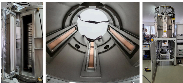
Fig. 12. The magnetron sputtering facility C.I.D., installed at the CERN MPT Workshop. C.I.D. is used to prepare the base material for the amplification stage of the detector by sputtering DLC on Apical ® foils.
