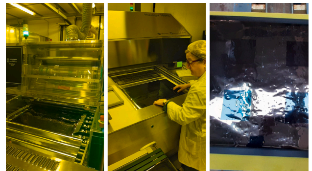
Fig. 14. DLC foil lamination with phot-resist film (left); UV exposure of the photo-resist by means of a Laser Direct Imaging (LDI) UV machine (center); DLC foil after photo-resist developing (right).
