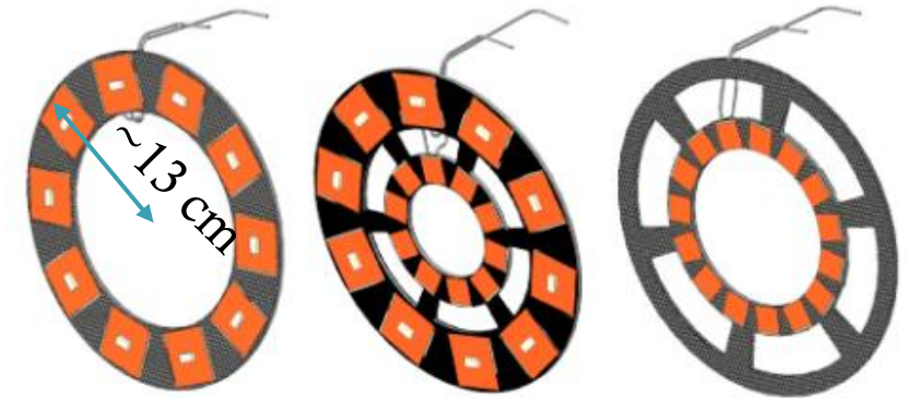
Inner system endcap rings (radius from ~5 cm to ~13 cm)
