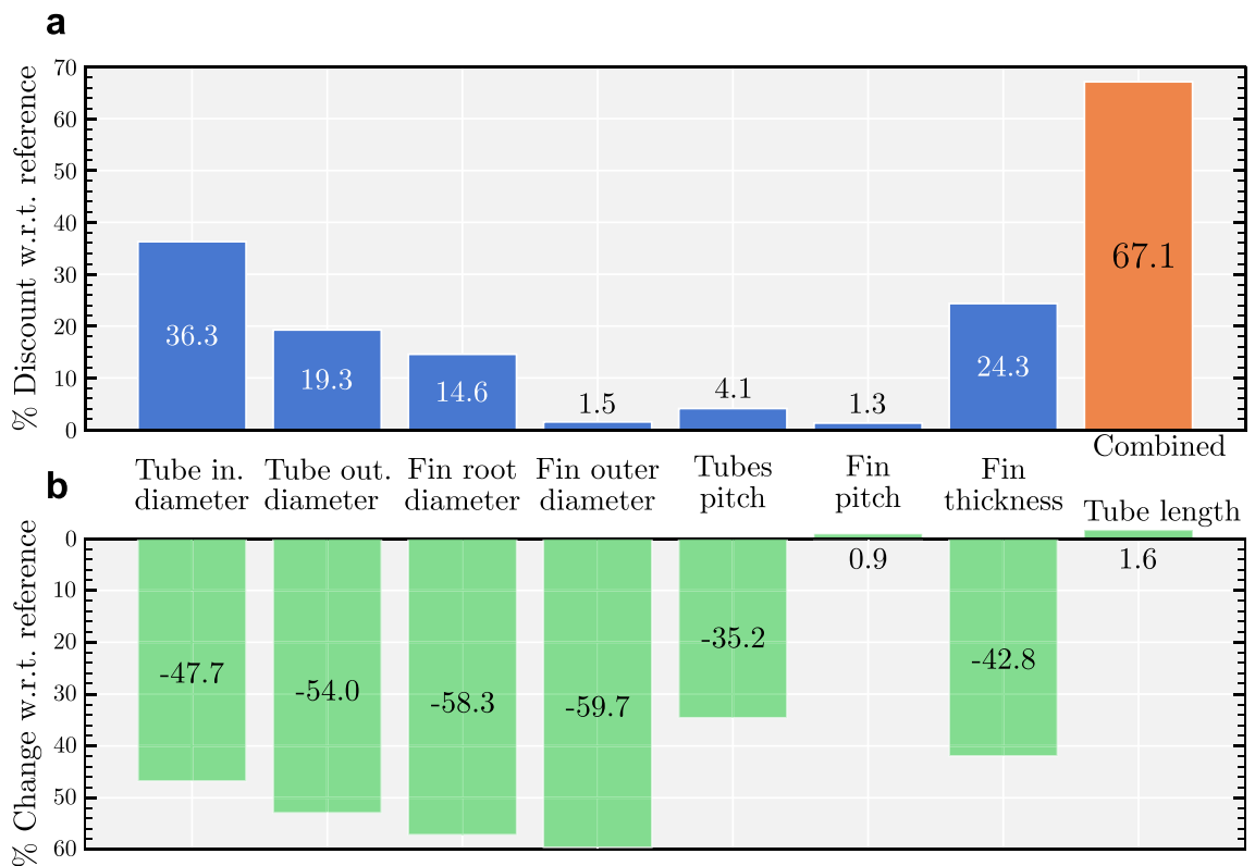
Figure 8. Cost sensitivity of different parameters and summary of the differences between the reference and the fully optimized designs as per Table 2. (a) Cost sensitivity of each parameter in terms of percentage discount w.r.t. reference design. This is calculated by changing one parameter at a time to match the optimized value found by the optimization process while keeping the others fixed to their original reference values, as in Table 2. The difference in cost is then computed with respect to the reference design and presented in this figure. (b) Relative change between the optimized and reference design parameters.
