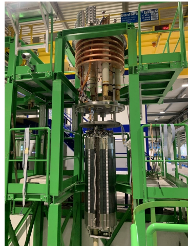
Fig. 22. Cross-section of the recombination dipole (right) and short model in the test station.
