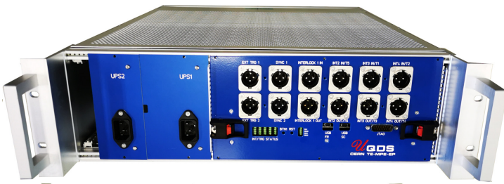
Fig. 7. UQDS v2.1 crate serving as the baseline prototype for the 11 T dipole (MBH) quench detection system. The crate is not equipped with top covers to illustrate its construction.
