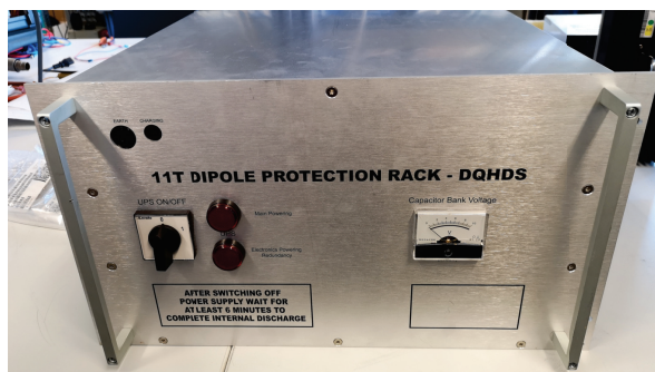
Fig. 6. QHDS for the protection of the 11 T dipole (MBH) magnets.
