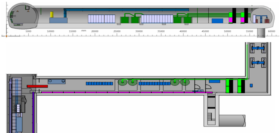
Fig. 11. Schematic of the RF system layout (four per IP side) in the underground cavern above the LHC tunnel lateral view (top); and top view (bottom). The amplifiers and transmission lines are shown in green routed towards the tunnel located towards the right.
