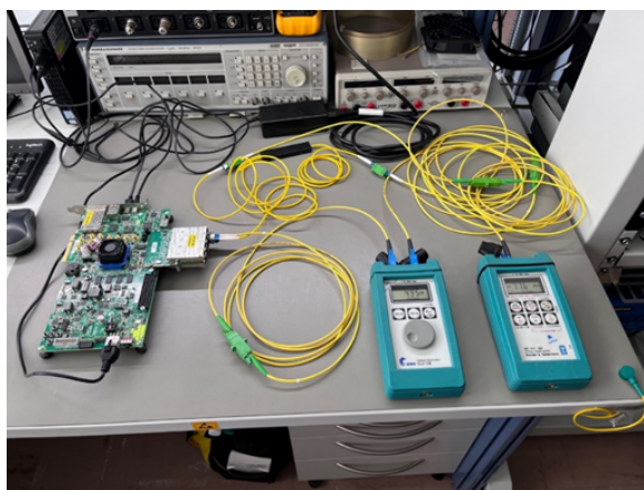
Figure 3. Image of the offline measurement setup for the Rx sensitivity test.
