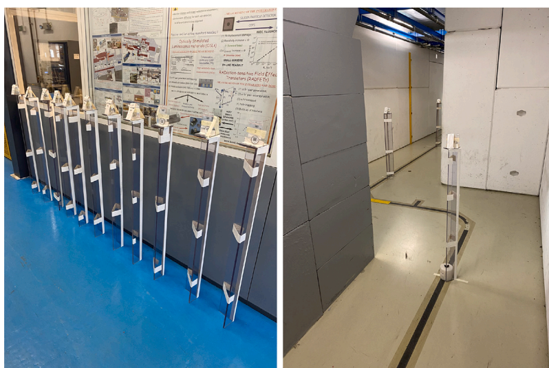
Fig. 5. Photos of the activation detectors: detectors mounted on the PMMA supports before the installation (left), view of the detector 10, 7, and 8 in the access maze (right).
