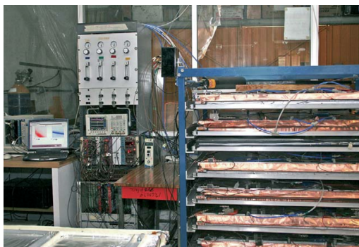
Fig. 5. (Right) The muon tracker at UNAM laboratories with a readout system. (Left) Schematic view of the muon tracker.
