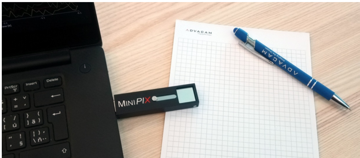
Figure : Minipix-EDU connected to a laptop. Taken from: https://www.linkedin.com/pulse/fascinating-patterns-drawn-radiation-particle-physics-jan-jakubek/
