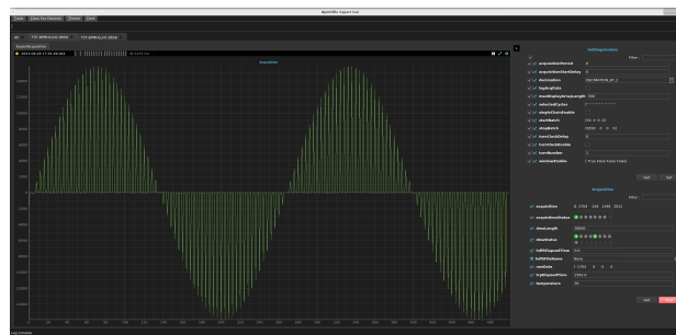
Figure 3: A screenshot from the expert GUI application. The expert settings are listed on the top right corner. The acquisition plots show data from the lab setup where the output of a pattern generator configured to produce sinus waves, is connected to one of the ADCs in order to verify the system.
