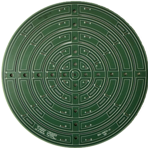
Fig. 7. Newly designed PCB transducer for the AD cooler.
