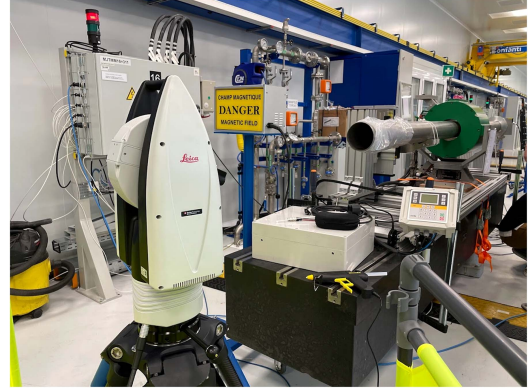
Fig. 5. Measurement setup used for the experimental validation. In green, the solenoid magnet.
