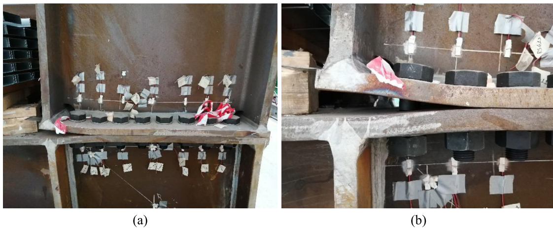
Fig. 26. Joint C2 at end of test: (a) general view of the connection; (b) detail of bolt rows 1 to 3.
