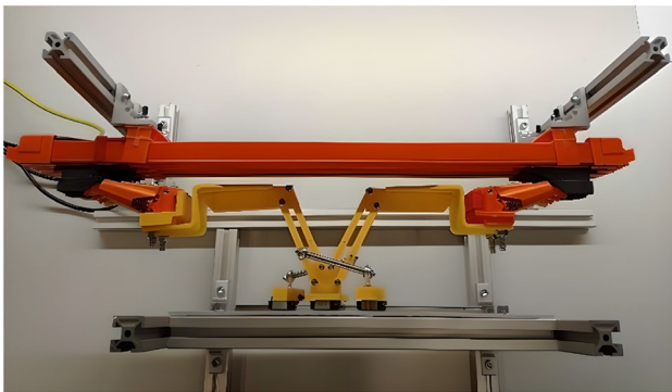
Fig. 20 Prototype made of 3D-printed components (top view)
