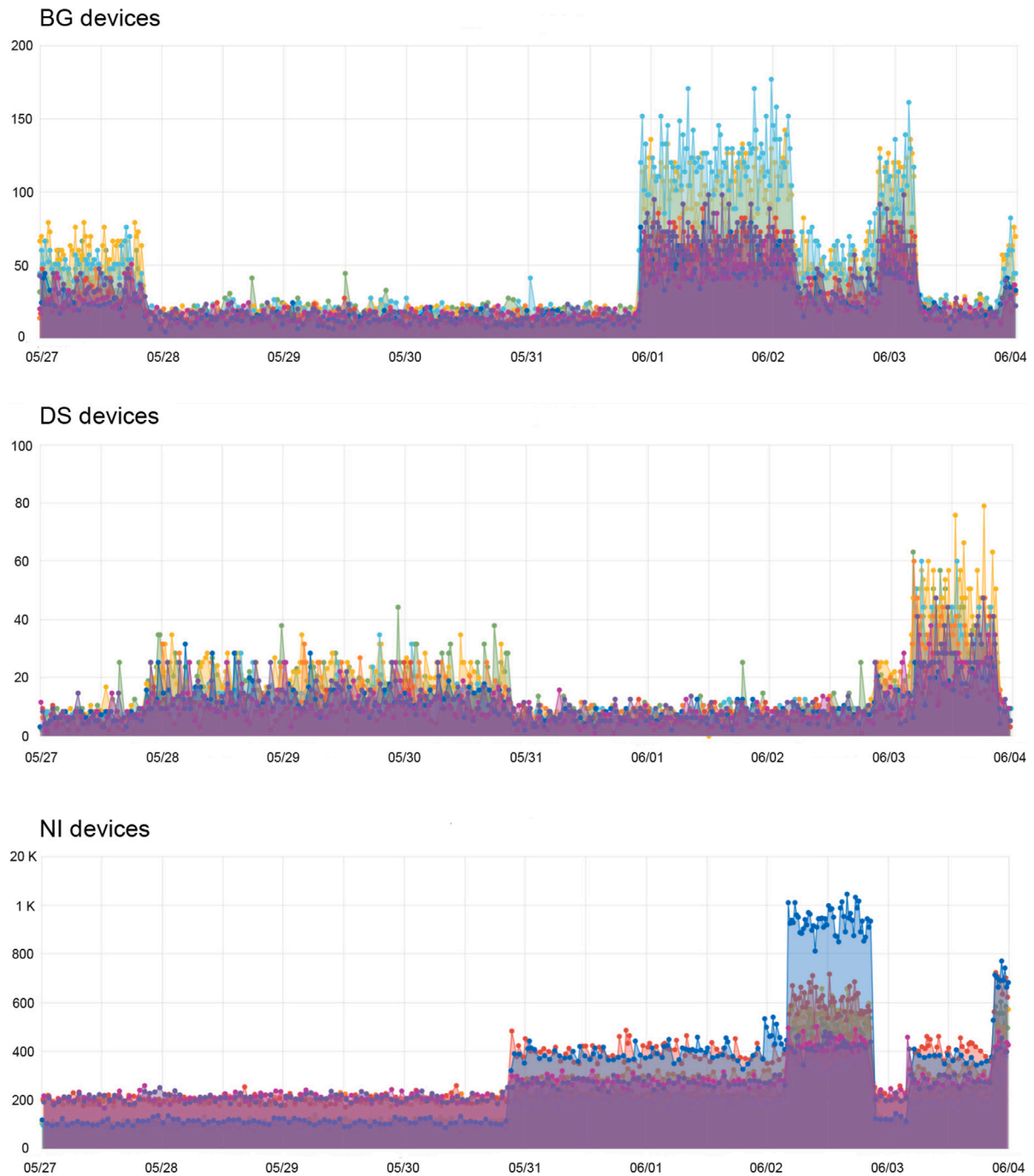
Fig. 7. Monitoring tool output showing the normalized rate for the period of the precise placement tests for BG, DS and NI devices respectively. Each subfigure shows the eight devices used in different colors. Notice that some of the samples were undoubtedly detected by the W-MON system while other samples with lower activity were not able to trigger the alarm by exceeding the threshold. Tables 2–4 show the detailed results.
