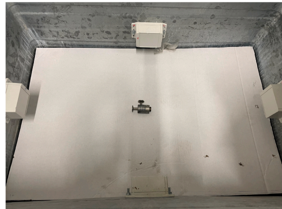
Fig. 6. An example of how the radioactive samples were placed inside the containers, on top of the cardboard. Below the cardboard the container is filled with the PPE.
