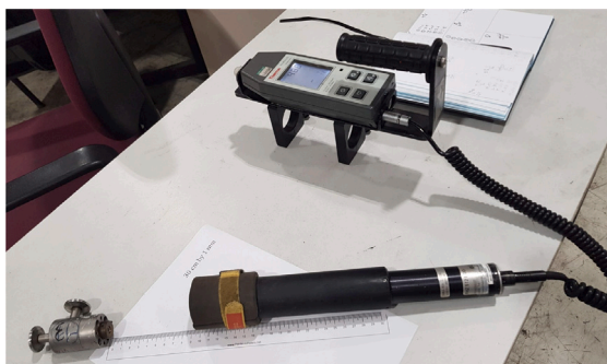
Fig. 5. The measurement procedure with the BGO survey meter. The photo shows the measurements performed around the sample, on all its sides to take into account the non-uniformity effect which was observed. The position, angle and sample remained the same in each measurement.
