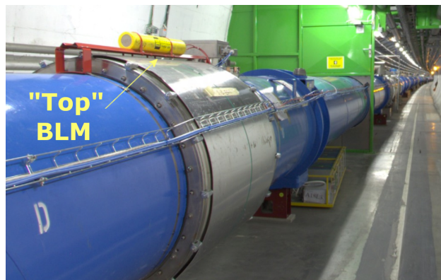
Figure 1: BLM installed in an LHC arc sector on top of the interconnection between the LHC dipole magnets. Each arc half-period contains 2 BLMs installed on top of the dipole interconnects, and 4 BLMs in the vicinity of the LHC quadrupole magnets.
