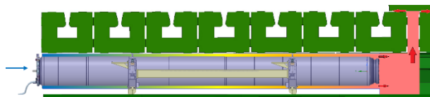
Figure 5: Example of an improved cooling system design using annular sleeve and chimney at rear of shielding
