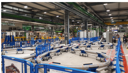
Figure 6: Superconducting Link at CERN in SM18.
