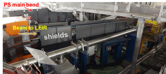
Figure 1: Part of the ITE line from Linac 3 to LEIR. Magnetic shields have been installed to reduce the stray fields from the close-by PS main bend. Beam travels from left to right.
